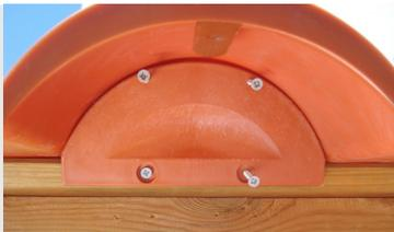
1. Anti-bird closure: The tile is fixed to the structure by placing 2 screws on the inside arch of the panel and 2 screws on the batten. This anti-bird closure holds the first line of tiles to the structure of the building, avoiding exposed screws on the roof. 4 pieces/lm
